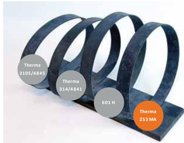
Therma 310S/4845 and Therma 314/4841 rings collapsed due to their own weight. 1000 °C/1830 °F, 35 hours, 1 mm/0.04 in thickness.
